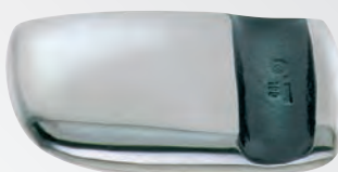
5 Low Crown Dollies sole pattern, face curved to all sides face 106 x 60 mm, height 25 mm, 950 g Art.No. 0190010000
