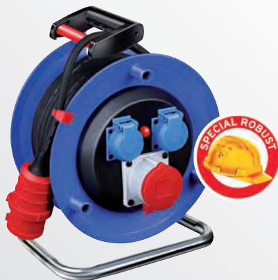
6A Garant® CEE 1 Cable Reels 1 CEE-plug 400 V/16 A, 2 water-jet protected sockets 230 V/16 A, 1 CEE-socket 400 V/16 A: earthed sockets connected to separate phases
