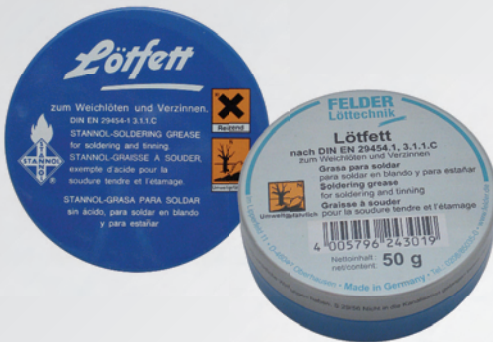
4 Soldering Paste (Grease) for soldering tin-plate, leaded shett and for tinning copper and brass DIN 29454-1 3.1.1.C not suitable for electrical engineering and electronics.
