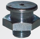
5 M1 Button Head Grease Nipples round head, hexagon version, galvanized C: Ø 16 mm, SW: 17 mm
