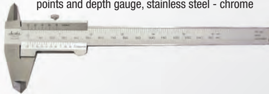
7 Pocket Slide Calipers open slide, monoblock, fully hardened, 4-way with cross-points and depth gauge, stainless steel - chrome
