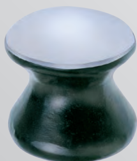
13 Dollies "Diabolo" face 60 mm dia, height 55 mm, 850 g Art.No. 2004010000
